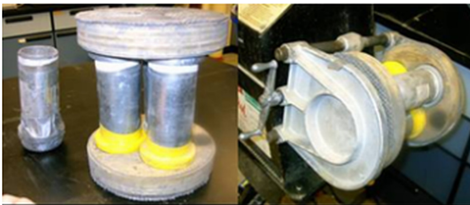
Fig. 1. Scaled-up milling procedure using Red Devil 5400 Twin-Arm Paint Shaker.
